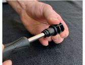
3. To unclog the nozzle, use a screwdriver to remove the Governor from inside the PX55 nozzle.
