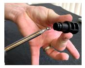
**5**. If necessary, remove any build up. Replace Governer in nozzle
