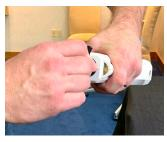
**1**. To determine if your nozzle is clogged, use nozzle wrench to remove the PX55 nozzle from the sprayer.
